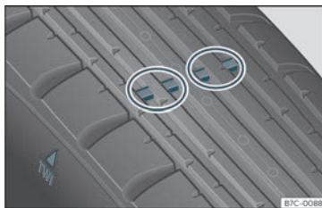
Fig. 213 Tyre profile: tread wear indicators.
