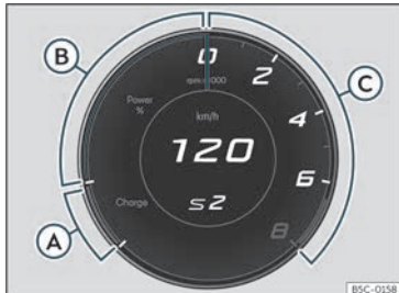
Fig. 57 Digital instrument panel: Powermeter (Cupra view)
