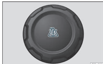
Fig. 207 Engine compartment: coolant expansion tank cap.
