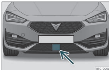
Fig. 148 On the front bumper: radar sensors.
