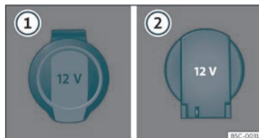
Fig. 129 12 volt power socket: ① inside the front armrest, ② in the luggage compartment.
