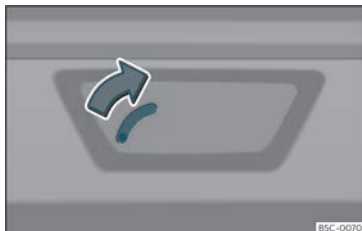
Fig. 85 Detail of the luggage compartment: emergency unlocking
