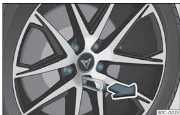
Fig. 35 Wheel: wheel nuts with caps.
