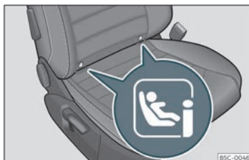
Fig. 28 Front passenger seat: ISO-FIX/i-Size securing rings.
