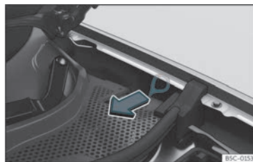
Fig. 194 Between the left wing panel and the engine bonnet hinge: Charging connector manual release mechanism puller.
