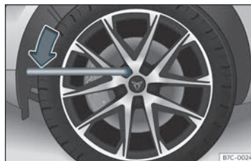
Fig. 37 Wheel change: loosen the wheel nuts.
