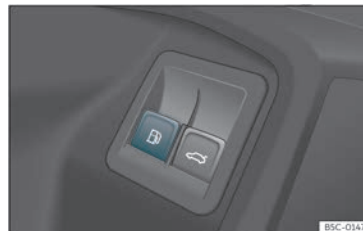
Fig. 198 Driver's door: tank flap release.
