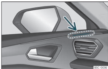
Fig. 174 Door: warning lamp
