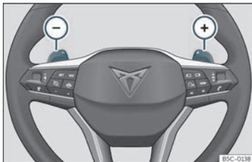
Fig. 146 Steering wheel: automatic transmission levers
