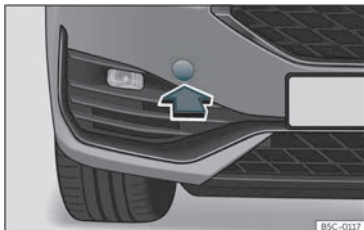
Fig. 43 On the right side of the front bumper: remove the cover.
