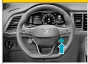
1. Press start and stop button if the vehicle is fitted with a "keyless entry" system.
