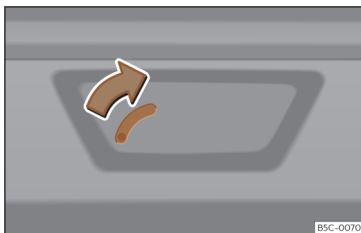
Fig. 80 Luggage compartment: manual release.
