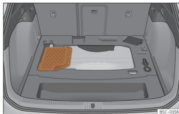
Fig. 219 Hybrid vehicles (PHEV): location of the battery in the luggage compartment
