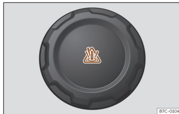
Fig. 212 Front compartment: coolant expansion tank cap.
