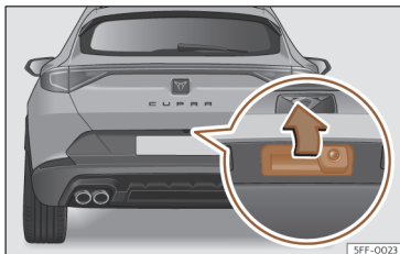
Fig. 75 Rear lid: opening from the outside.
