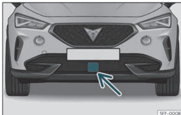
Fig. 140 On the front bumper: radar sensors.
