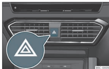
Fig. 87 Dash panel: hazard warning lights switch
