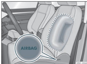
Fig. 21 Side airbag in driver's seat.
