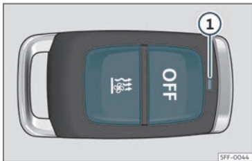
Fig. 125 Auxiliary heating: radio-operated remote control.
