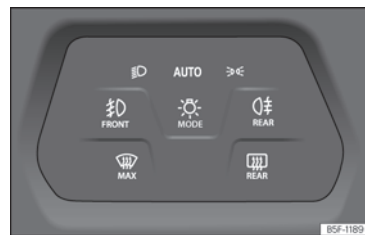
Fig. 85 Dash panel: lights control.
