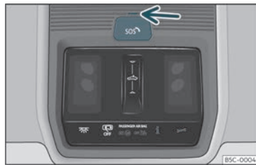
Fig. 32 On the roof console: voice service controls
