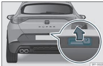
Fig. 77 Rear lid: opening from outside.
