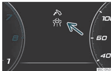
Fig. 54 Eco-efficient driving assistance indication (schematic representation).
